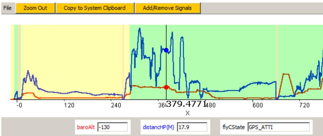
Here, the value tracker is currently at time 379.477, baroAlt has the value -130, and distanceHp has the value 17.9. The state signal flyCState has the value GPS\_ATT1.
